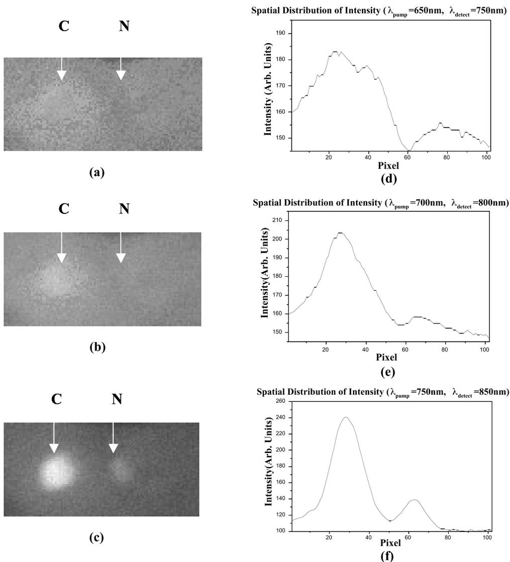
**Figure 5:** Contrast agent emission images of a prostate cancer-and-normal tissue sample recorded at (a)  $\lambda_{\text{pump}}=650\text{nm}$  and  $\lambda_{\text{detection}}=750\text{nm}$ , (b)  $\lambda_{\text{pump}}=700\text{nm}$  and  $\lambda_{\text{detection}}=800\text{nm}$ , and (c)  $\lambda_{\text{pump}}=750\text{nm}$  and  $\lambda_{\text{detection}}=850\text{nm}$ , with a perpendicular polarization configuration; (d), (e), and (f)
