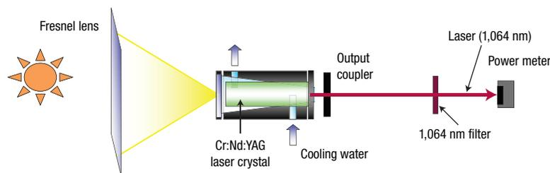
**Figure 2** A schematic of the solar-powered laser design. A high-performance 1.3-m<sup>2</sup> Fresnel lens collects the light and a highly efficient, broad-absorption-band chromium-doped Nd:YAG ceramic laser gain medium enables most of the Sun's wide spectrum to be captured.
