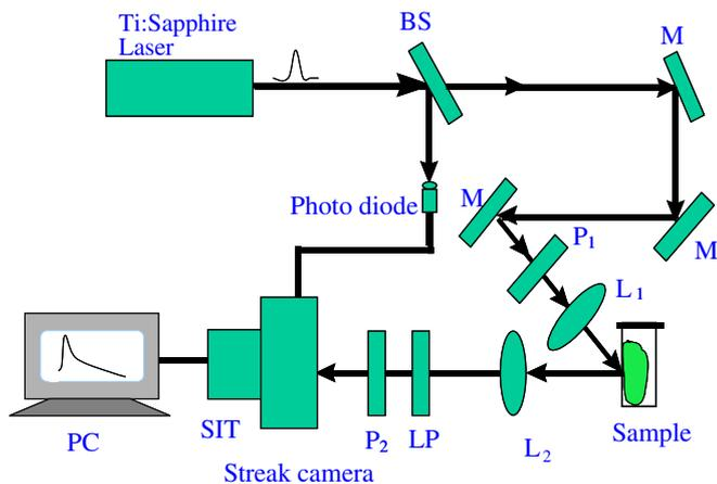
Fig. 1. Schematic diagram of the experimental set up used for time-resolved fluorescence measurements, where  $P_1$ ,  $P_2$ : polarizers; M: mirrors; BS: beam splitter; LP: long pass filter; L: lenses; SIT: silicon intensified target.
