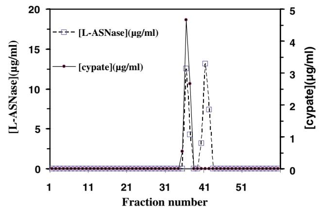
**Fig. 1** The elution profile of rude CY-ASP by gel filtration on Sephadex G-100 column. Fractions collected from the column were assayed for proteins content by the bicinchoninic acid (BCA) Method and cypate content as described in "Materials and methods"
