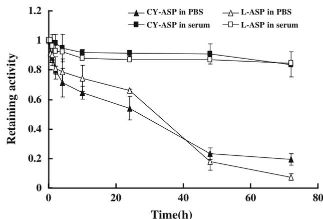
Fig. 7 Retention of L-ASNase activity in the presence of 20% DMSO in PBS and blood serum at  $37^{\circ}\text{C}$ . The relative activity equaled to the ratio of every activity value to the highest one in the same curve
