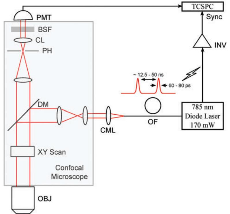
Fig. 1. Schematic of the FLIM system. OF, optical fiber; CML, collimator lens; OBJ, objective; DM, dichroic mirror; PH, pinhole; CL, collection lens; BSF, bandstop filter; INV, inverter.
